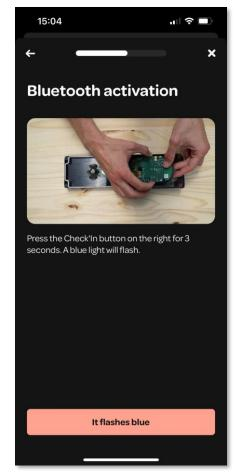
Press the button on the Check'In Infra for 3 seconds, then tap on 'It flashes blue'
