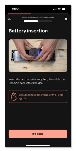
Insert the two provided batteries, ensuring to respect the polarities (+ and -)
